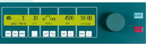
ROTO SILENTA 630 RS control panel: Entry of the parameters is exact, fast and easy with selector keys on the foil keypad and the adjusting knob.
