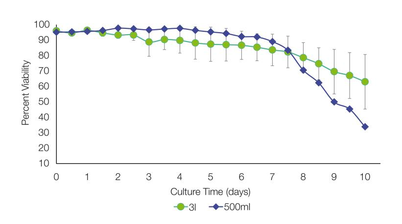
Temp: 37°C | pH: 7 | C<sub>L</sub>= 40%sat | Cell line: CHO DG44 | Seed D: 0.3x10<sup>6</sup> cell/ml | Media: PROCHO5 (supplemented) Complete media | Impeller: single marine impeller | Sparger: Micro-sparger: Aeration | DO control (maximum 0.007 VVM)
