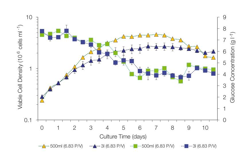
VCD (triangles) and glucose concentration (squares) of 500ml and 3I bioreactors run at center point P/V conditions. Three 3I bioreactors and one 500ml bioreactor were run at center point for 10-day fed-batch processes. Error bars are one SD for the 3I runs.
